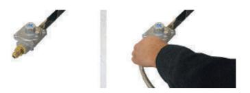
After orifice has been tightened attach flexible hose
