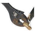
Turn propane valve counter-clockwise to loosen
