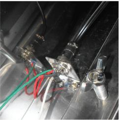
LOCATION OF SCREWED-IN CONNECTION POINT THAT LEADS TO AC ADAPTER
