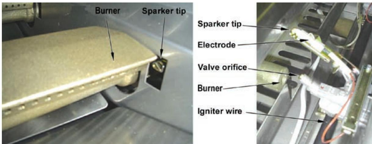
**Problem: Burner tube is misaligned over the orifice**
