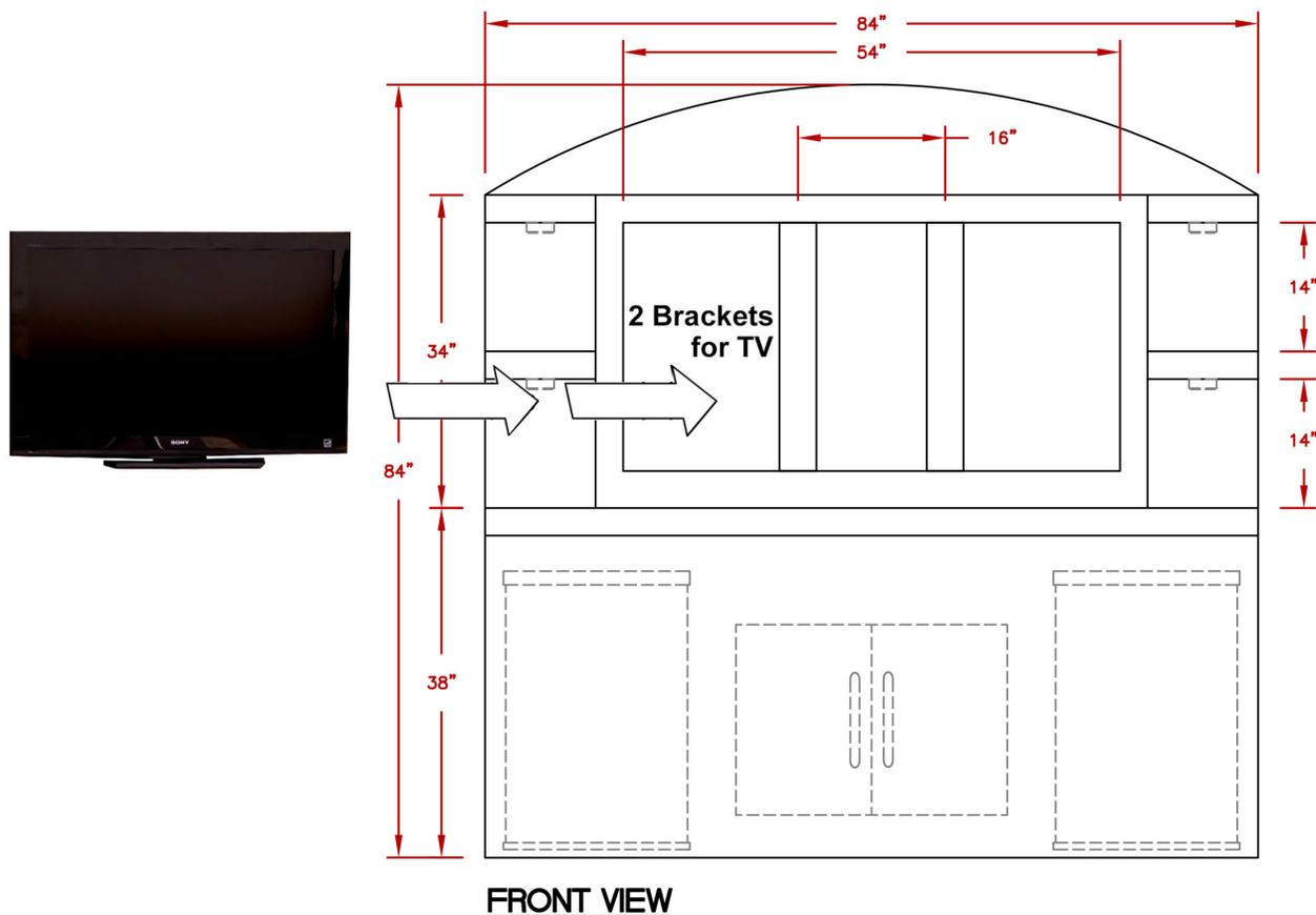
The television enclosure is 54" Wide by 27" Tall. Please note that diagonal screen measurements will not give the true physical dimensions of the television because the diagonal measurement does not take into account the television's housing. Therefore, the best measurement to use is the actual height and width of your television (including the base if used).
