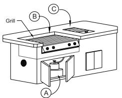
B Then take other end of "T" adapter with hose attached and connect to end of male located underneath and at the back of the grill. (Use gas rated tape seal on all connections).
