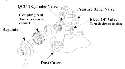
Place the dust cap on the cylinder valve outlet whenever the cylinder is not in use. Only install the type of dust cap on the cylinder valve outlet that is provided with the cylinder valve. Other types of caps or plugs may result in leakage of propane.
